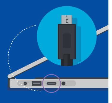
USB-C connectors and cables support USB 3.1, the current industry standard protocol<sup>2</sup> for Universal Serial Bus (USB). It is the fastest USB standard protocol to date, saving file transfer and backup time with data transfer speeds of up to 10 Gbps. USB 3.1 can work through USB Type-C connectors, but it's backwards compatible with older USB connector styles like A and B.
