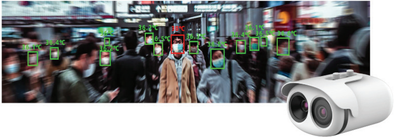
Figure 6: CohuHD Non-Contact Thermographic And Facial Recognition Camera
